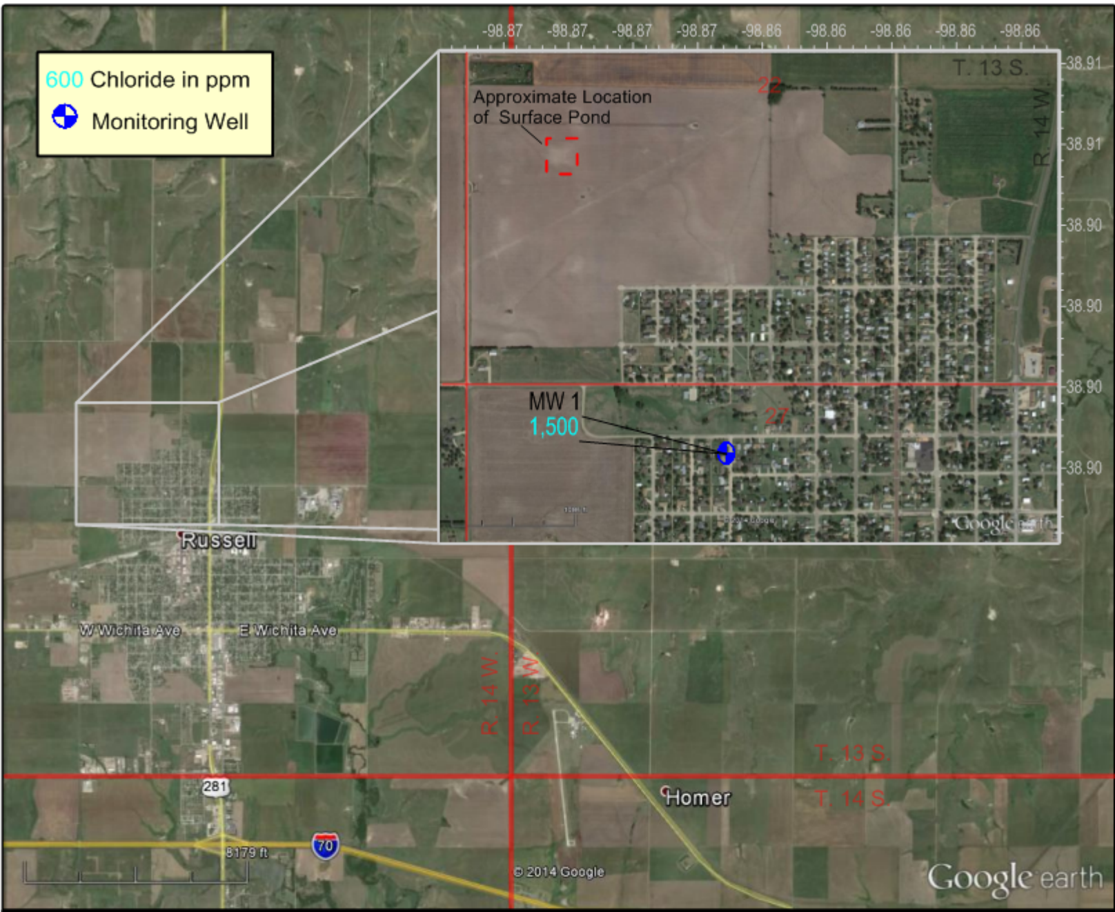
City of Russell Groundwater Monitoring Site Sections 22 and 27, Township 13 South, Range 14 West, Russell County, Kansas 2016 Groundwater Chloride Levels District #4 - Sampled 10/28/2015 - Map Drawn on 10/29/2015 by C. Neeley Kansas Corporation Commission
