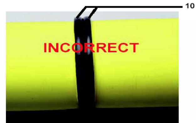
10. Excessive heat time or pressure applied during heating; melt bead too large
